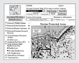
OPIS online mapping application displays bottom types in a marine protected area in North Carolina to assist in determining the suitability of the site for disposal of ocean-dredged material. Box 4.2 continued
